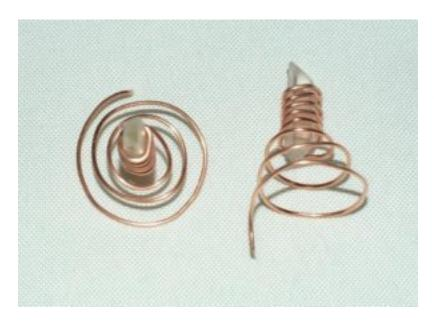
the small end of the coil around the middle of the crystal. Remember that the whole thing will have to fit easily in the pipe. You may want to tape or glue the coil to the crystal so the unit doesn't fall apart when you drop it down into the pipe.
