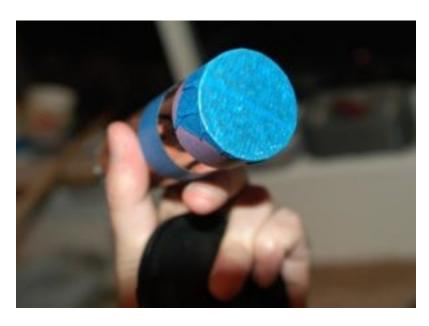
2. Thoroughly tape one end of each pipe closed. If you're not thorough, resin will leak out the bottom.
